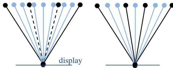
**Figure 7. Two configurations for 4 transmitted views, and 9 displayed views. Solid black: transmitted views that can be mapped directly on an output view. Dashed: transmitted views that cannot be mapped on an output view. Light blue: interpolated view.**
