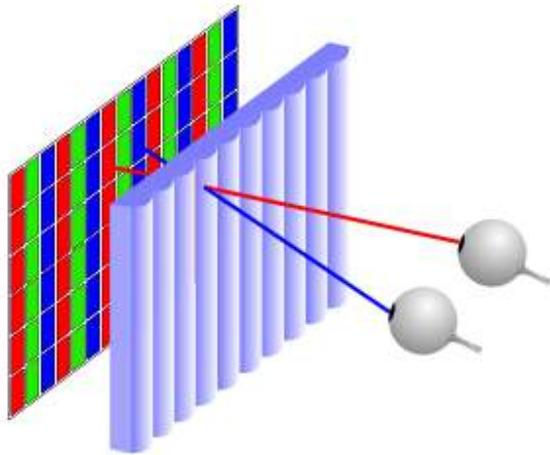
**Figure 2. The auto-stereoscopic lenticular screen. The various sub-pixels are refracted to different angles by the sheet with the lenticular cylindrical lenses. In this way the left and the right eye are presented with different views.**
