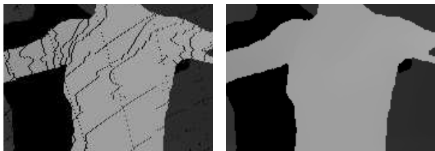
(a) Warped depth map before median (b) Warped depth map after median
